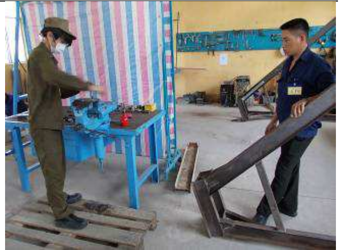
Photo 20: Tapping M20 by hand. This gives strength.
