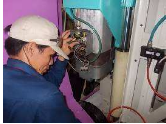
Photo 3: Our teacher Jerry sits in the vertical lathe and wiring the terminal box. For weeks we were looking for the parts. They learned only good disassembly allowed and good assembly.
