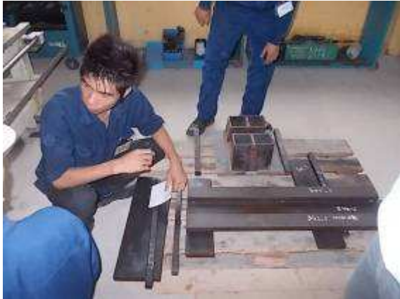
Photo 42c: The 2nd Cross slide of DM2 S is now being prepared for welding. Moreover, the drawings improved.
