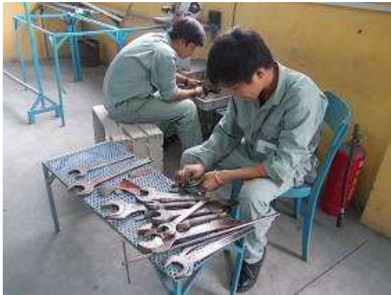
Photo 12: Here we have some tool that are not stainless. The rust is a big problem in Vietnam, we have to decide, many tools to protect against rust with paint.
