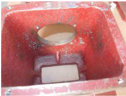
Photo 12: That, everything is edited are also cleaned, do not know our apprentices. Contamination. Not properly deburred is even not satisfactory.
