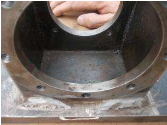
Photo 13: The case of the new LC is 5 system. Unfortunately not well plastered. 0.5 mm edge breaks we need to practice more intensively.
