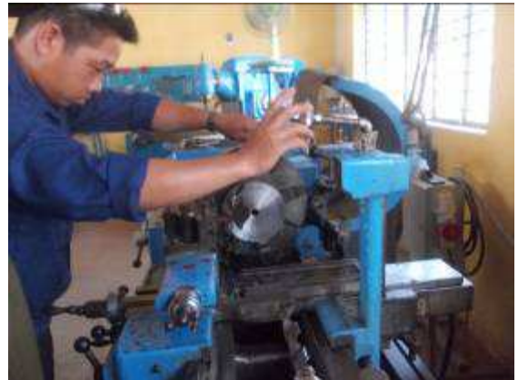
Photo 29: A19 apprentice was already in the army. He turns here a flange on the Swiss Menziken lathe.
