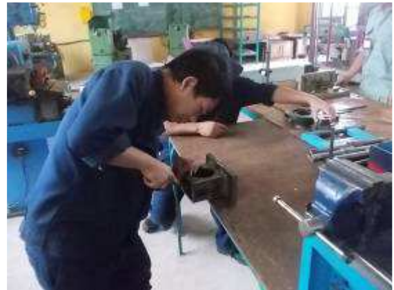
Photo 9: The Apprentice A 24 deburred, the metal housing of the expansion plant WIAP LC 05 With the deburring we have a little trouble in Vietnam. The trainees and the teachers do not see the reason , for what that is.
