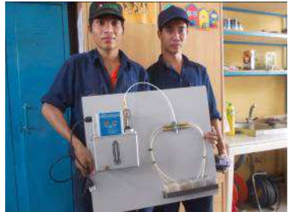
Photo39: The teaching must go on. So that our boys learn something for the future. Here was made a test station for impulse lubrication for machine tools
