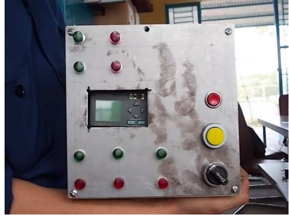
Photo 20: Here the apprentice A18 has a pattern made for the tropics Cabinet Control controller TCC. We will make 6 pcs for Luanda and Cabinda and 8 for 4 pieces in stock. This is just the final exam.
