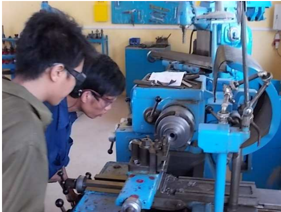
Photo 22: The Apprentice turns a flange for metal expansion plant Wiap LC 05 We have launched 3 pcs. Each plant with about 20 positions. Some apprentices have something to do.
