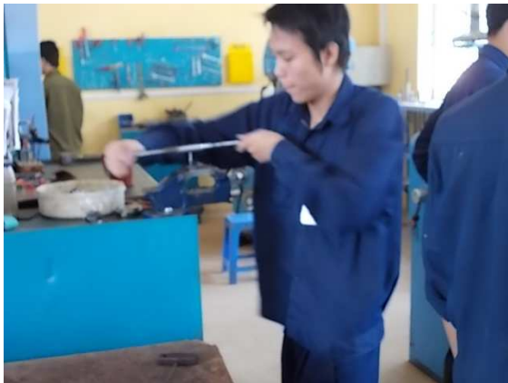
Photo 12: We need perforated plates with many threads, M6, M8, M10. The muscles are where all must be done by hand.
