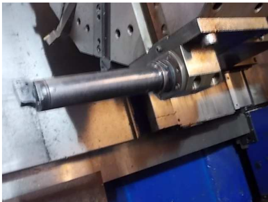
Photo 7: These holders were appointed by Sandvik, which are not stable.
