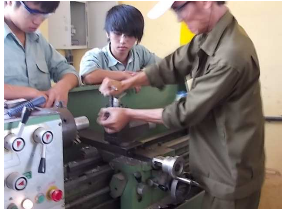
Photo 9: make 30 spacer rings in various lengths with parting, here's the job. That's what it all now B and C apprentices.
