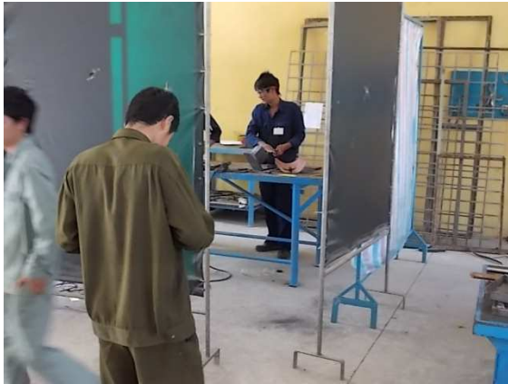
Photo 18: Our welding walls take them off and just go away. Especially the teachers then weld. Without regard to third parties, and whether they are blinded. We will distribute to those negative points, which allow this in the future.
