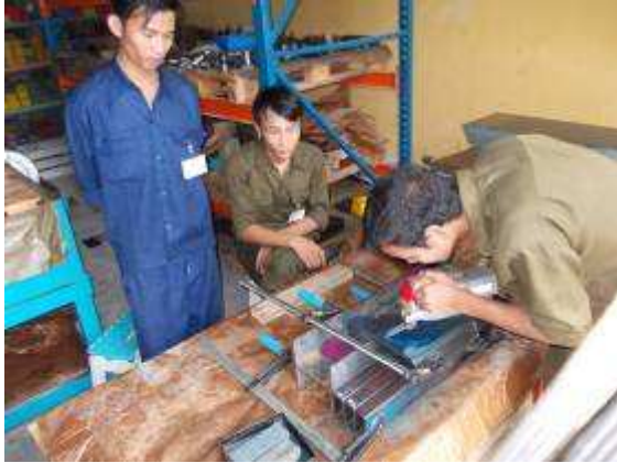
Photo 9: For our first CNC lathe that we build in the school, the WIAP DM2S is here the turret console scraped.
