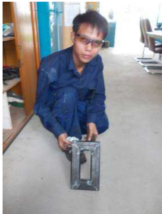
Photo 8: For the audit we have made 16 such 4-square tube frame. To see if the trainees can weld within 1 mm. 90% was ok.
