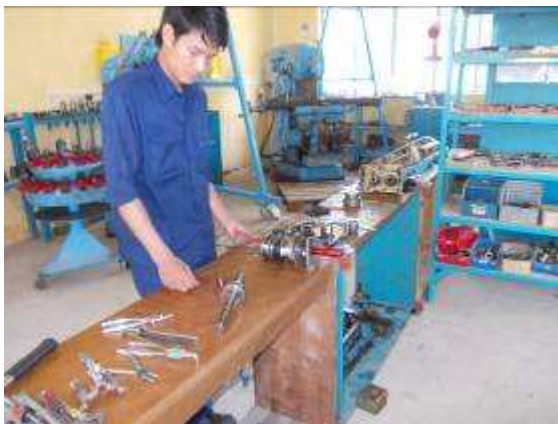
Photo 5: When disassembling is important to lay everything properly for reassembly. Each spacer is to be re-installed in the right place. A12 does a very good job here.
