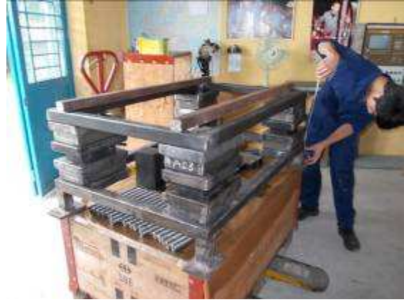
Photo 7: Here we build a vibrating table, which is equipped with 8 rubber dampers.
