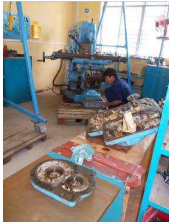
Photo 4: All the feed gear is broken.
