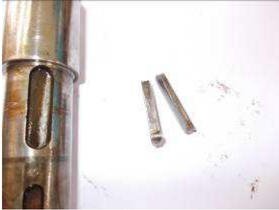
Photo 4: Only after almost everything was dismantled, we could find the sheared wedge.
