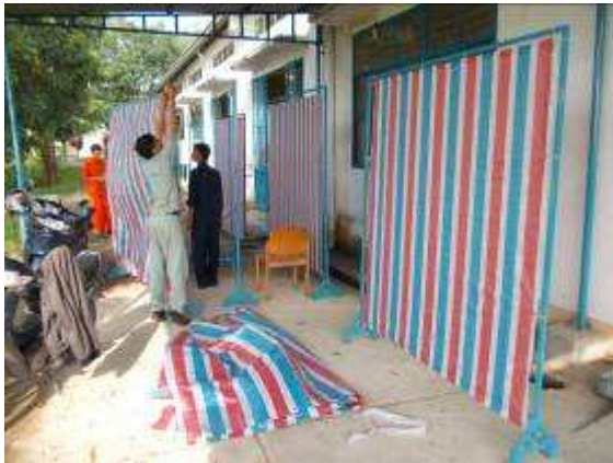
Photo 16: barriers between the machines that prevent chips, light welding, grinding dust endanger the neighbours. Everyone who works at a machine, is now responsible for ensuring that he does not endanger others.
