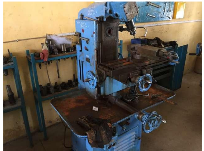
This Swiss milling Schaffner everything was rusty on the machine. Without coolant, Emulsion, work is not good, then the rust immediately. And let too long to act the rust eats into the steel, leaving indentations. Room 2 Photo WS10_80
