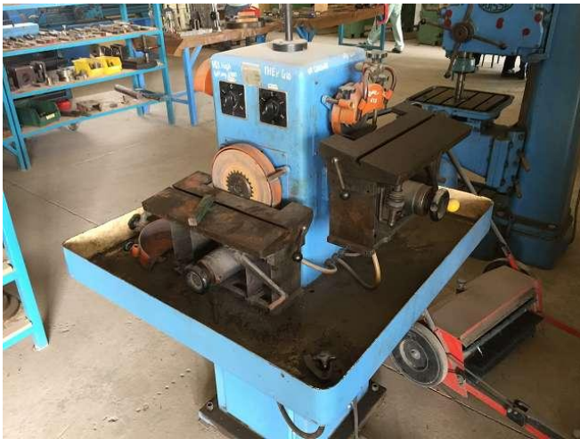
An exclusive tool grinder for 4 grinding wheels as well as diamond wheels was completely contaminated and unpurified in room 2 editing. Photo WS10_60
