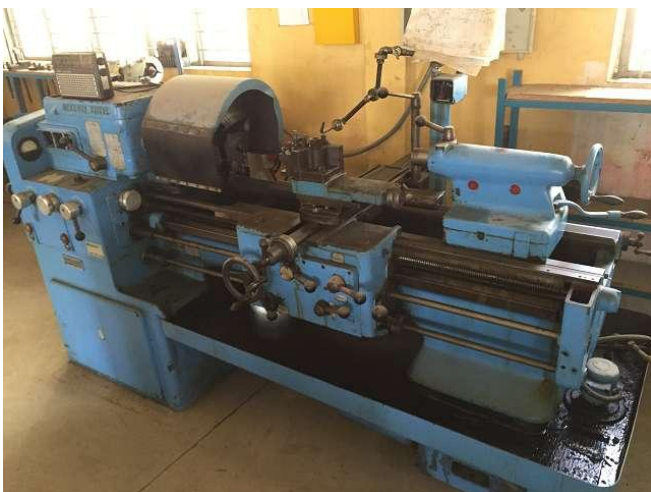
This valuable, old Swiss lathe Menziken from the canton Aargau was dirty and had no oil on the guides. We almost get tears while looking at the machines - state. Room 2 Photo WS10_70
