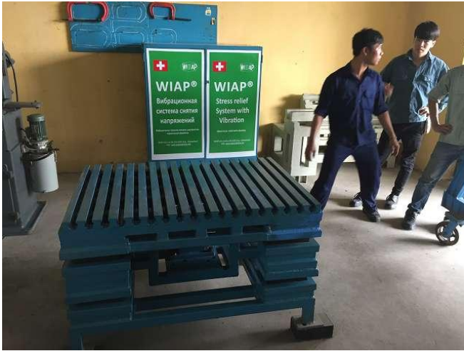
Welding shaker tables, 2 such we built in Vietnam. Unfortunately, the welds are not nice that we are the two never nehmen to Europe. We will leave the same table in Europe even calculate and still practice a little welding in Vietnam. Beautiful welding! Since we still have a task ahead of us. Space 1b. Photo WS10_570
