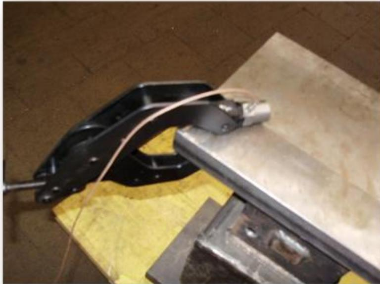
The measuring probe as it is mounted on the workpiece. Always use caution; the cable is very sensitive and should also not be "kinked".
