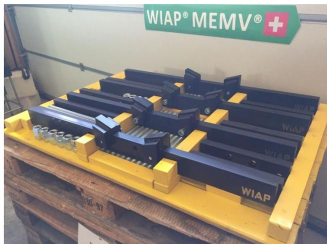
Mounting clamp set waves 400 to 800 mm
