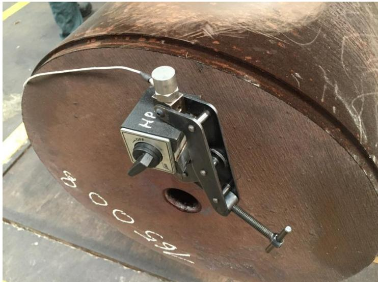
Photo: The measuring probe as attached to the workpiece
