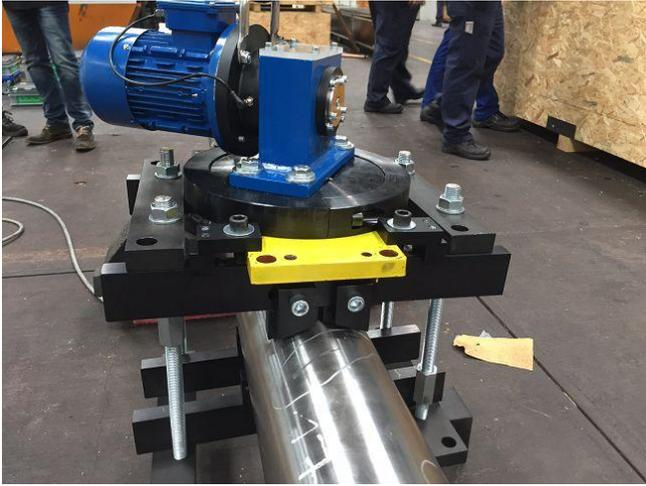
14. 4.22 prisms set for round parts up to 800mm
