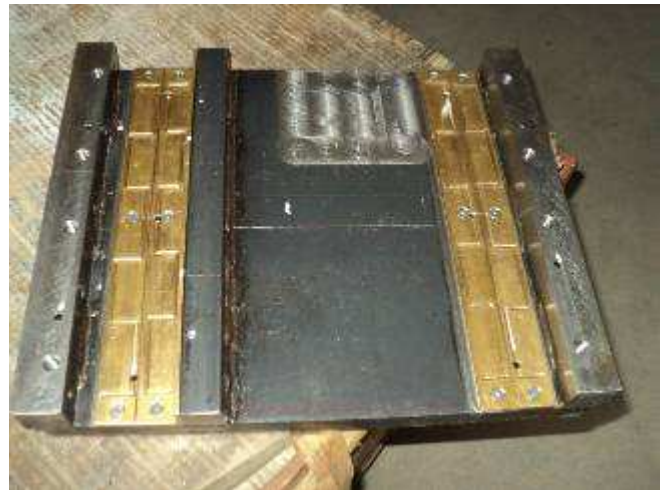
Photo 04: This slide has a lot of lubrication holes. We have now also decided a change so that more can be scraped. That's all good, the drawings will be changed immediately.
