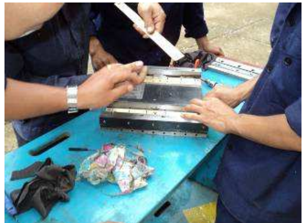
Photo 10: Since we have three compressors, compressed air is wonderful for the apprentices. But they have out in the open air, blow everything good and clean to prevent dirt particles get under the sliding surfaces. Slowly they realize that we are very attentive and have no tolerance.
