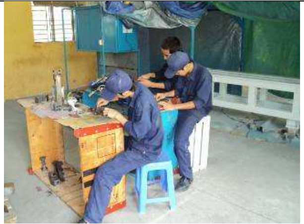
Photo 08: With great patience, they can sand the rust with sandpaper on the work pieces, which we prepare for painting.
