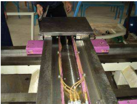
Photo 12: Here was placed the X carriage, now is scraped.
