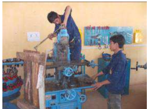
Photo 24: Here the apprentice Hieu, who was looking for the lube points and also had to lubricate. All oil lubrication are still marked with red. All lubrication points with yellow. For all machines have the Quick Start Guide are created with a photo of the key handling. Even the lubrication schedule for each machine will be created and the Draining an Spear parts plan . And everything is in the yellow box.
