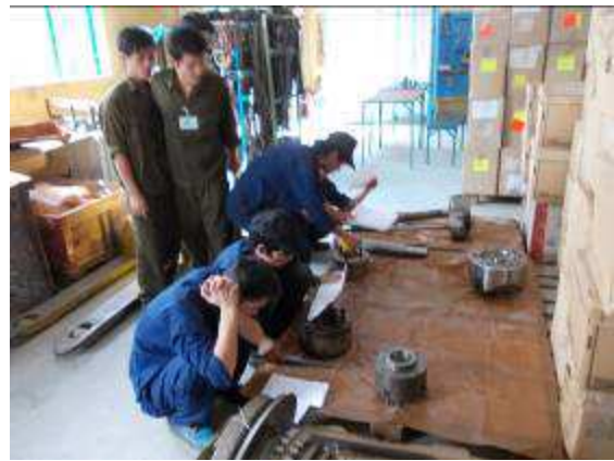
Photo 18: On the items are to write down the apprentices who have the spindle nose size because lying spindles, ASA 5? ASA 15? Long they studied the drawings.
