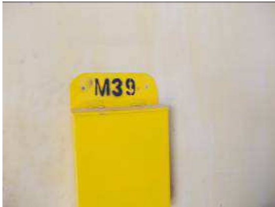
Photo 20: Since more than one year we've always wanted to introduce the yellow box system. Provided at each machine a box containing the maintenance schedules.
