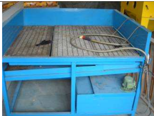
P31: This is our cleaning place, 1200 x 1200 mm. With water pump integrated. Our design. In room 5a, surface place.
