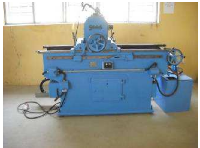
P16: German flat grinder, brand Göckel with 100mm length 1000 mm.
