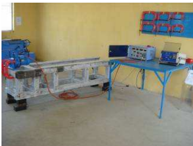
P23a: Stress relief area room 1 b. One old system and one new system is in function, for till 20 Tons work peace. In our place max. 1 ton possible.
