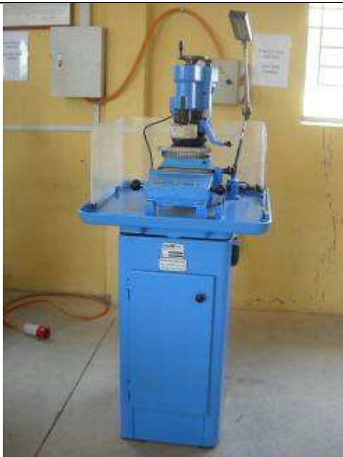
P17: Flat grinder "Hugi" Switzerland. Max 100mm.
