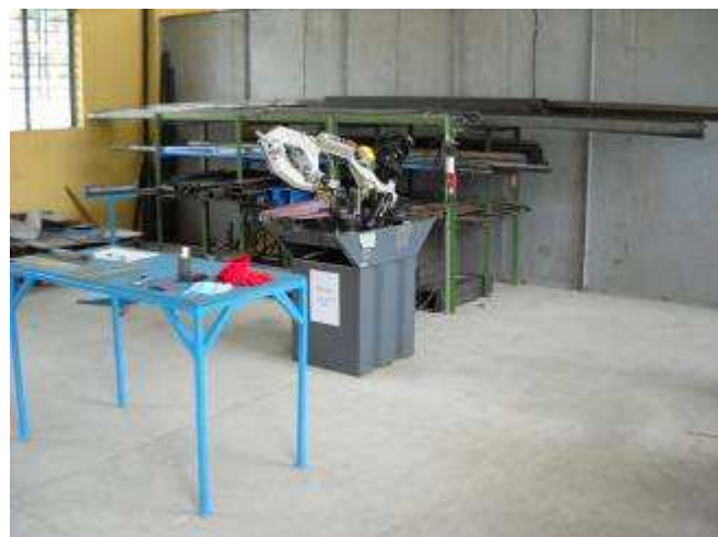
P26: Room 3a, material store with the bandsaw for 150mm size and 6 meter Length.
