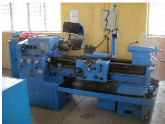
P11: These is our conventional lathe Menziken from Switzerland centre High 230mm x 1000mm.
