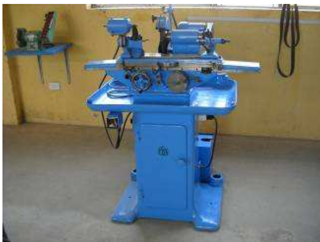
P18: Round grinder FST Germany, center high 75 mm length 300mm.
