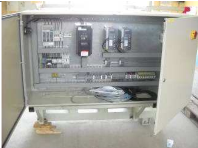
P5: Our electro cabinet for two DM2 machines.
