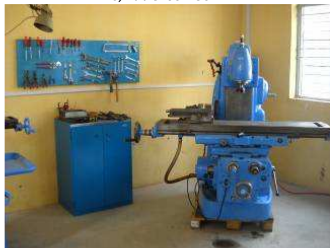
P10: Induma milling machine ISO 50, Table 300x1500 mm.
