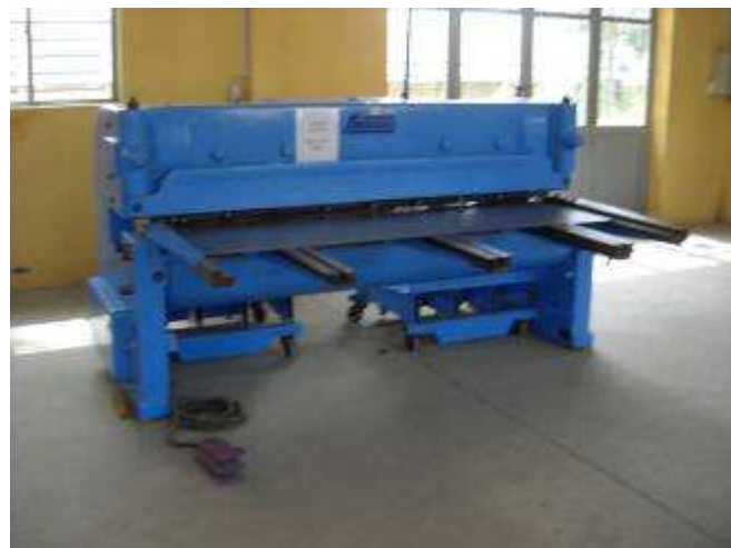
P20: Cutting machine Hänggi Switzerland 2mm( Max) x 2000mm.
