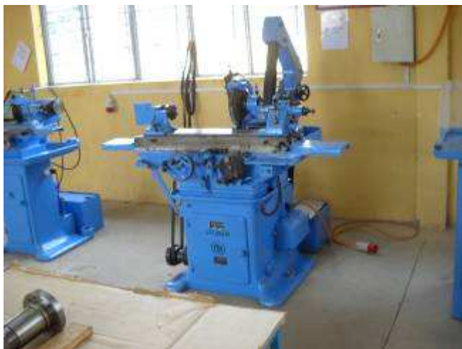
P19: Round grinder "Studer", length center high 110.
